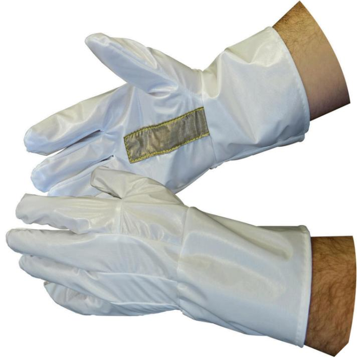
The E-Stat Gloves have continuous conductive strips that run from the inside of the palm to the outside surface of the gloves. This grounds the worker when using electrostatic spray paint guns and eliminates wrap back.
